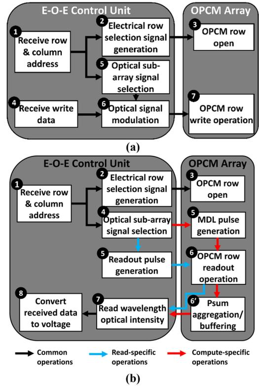
Fig. 4: Memory (a) write and (b) read operation in *OPIMA*; *OPIMA* utilizes multiple read signals simultaneously to perform computation operations. The differences in control flow between a memory read operation and performing in-memory computation are highlighted in (b).
