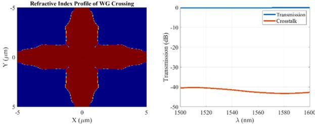
**Fig. 6:** Low-loss waveguide crossing designed with inverse design methodology (left) and its loss profile for C-band (right).
