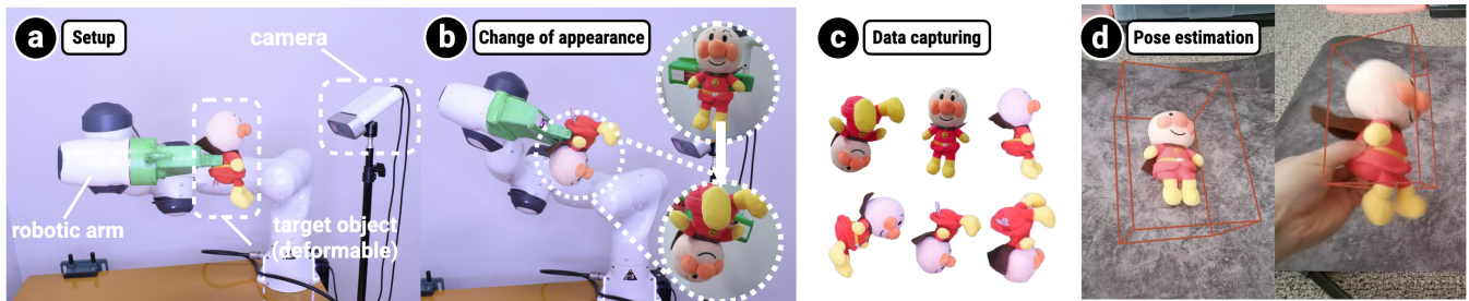
Figure 1: The RoCap pipeline is a robotic system designed to collect datasets for the purpose of pose estimation of appearance-changing objects, e.g., a deformable plush toy (a). The system consists of a robotic arm and an RGB camera, which allows for data collection (c) of objects with appearance-changing features (b). Through data augmentation and training on off-the-shelf deep learning models using the collected data, the system can effectively estimate the pose of the plush toy during manipulation, even as it transitions through deformation (d).
