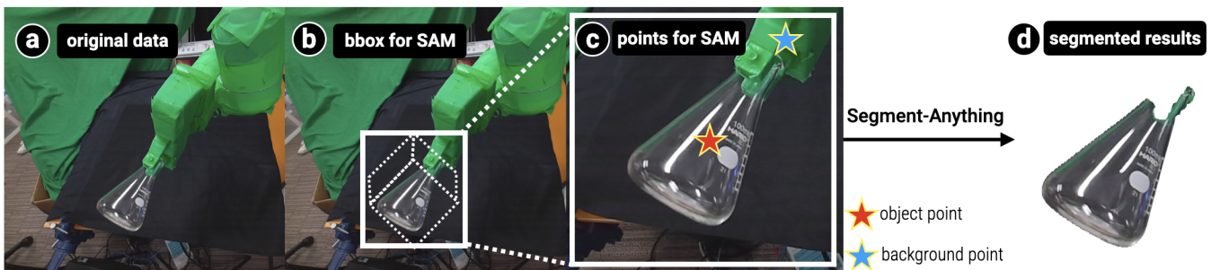
Figure 8: Data processing of data collected in by RoCap. RoCap generates mask for each image (d) by prompting SAM with bounding box (b) and points (c).
