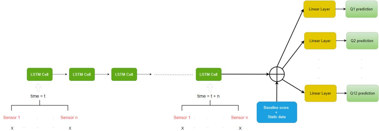
**Figure 4:** Architecture of the LSTM model used for predicting ALSFRS-R scores. The model processes time-series sensor data through sequential LSTM cells, capturing temporal dependencies. The output is combined with baseline scores and static patient data, then fed into multiple linear layers to predict each of the twelve ALSFRS-R sub-scores.
