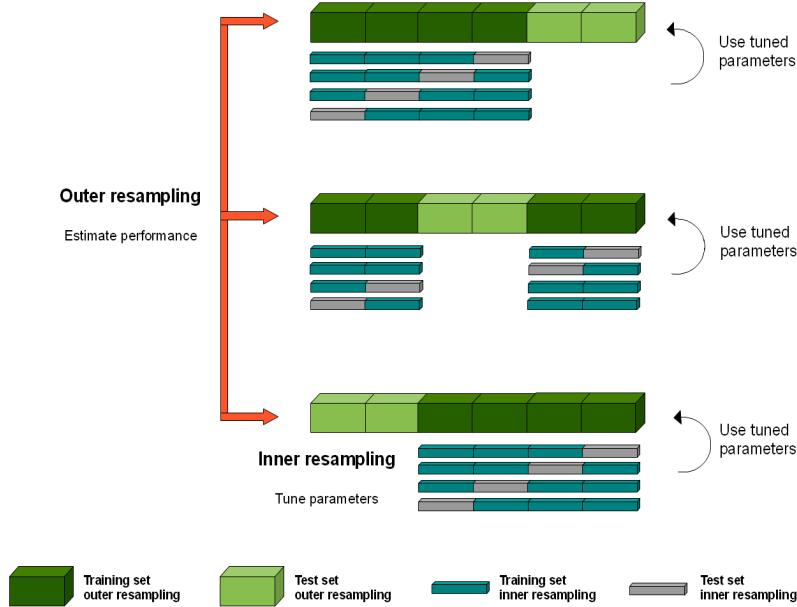
**Figure 3:** Cross-validation procedure for the hyperparameter tuning and final model fit in our work (Source: [20]). The original source illustrates the procedure without taking into account a grouped structure as in our dataset. Hence, in our work we adapted the procedure so that each patient’s complete data is contained in either the inner-train/test subsets, or the outer test-set.
