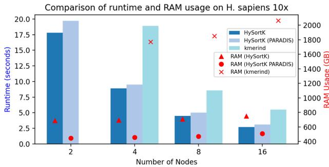
Figure 7: Comparison of runtime and memory usage between HySortK and kmerind [26] on *H. sapiens* 10x with  $k = 31$ .
