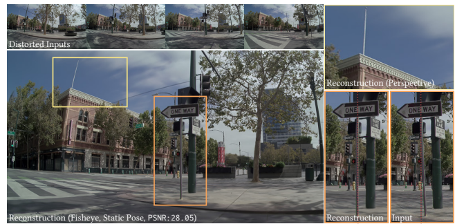
Fig. 17. AV Scene Reconstruction: Real-world AV and robotics applications often have to respect both distorted intrinsic camera models and are, at the same time, affected by time-dependent effects like rolling shutter distortions as frames are exposed at high sensor speeds. Our ray tracing-based reconstruction is well-suited to handle both challenges simultaneously, which we illustrated by an example of a side-facing top-to-bottom rolling shutter camera on an AV vehicle: the top inset (•) depicts faithful removal of the intrinsic camera model distortion by rendering with an undistorted camera, while the bottom inset (•) shows our ability to remove the apparent rolling-shutter distortions of the inputs by rendering from a static camera pose (linear indicators (•) exemplify the complex distortion of the inputs).
