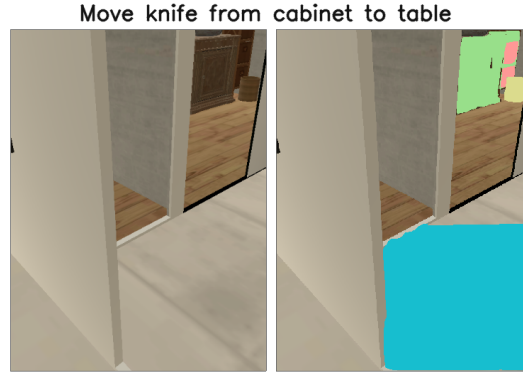
Figure 6: Example of an incorrect floor classifications. The floor is classified as a table (blue cluster), which is the end receptacle . The floor is filtered out in the UniTeam -agent, otherwise the agent would want to place the knife on there.
