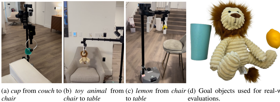
Figure 3: Examples of object manipulation from real-world experiments. The participant teams needed to find and move three objects (fig 3d) from the held-out apartment environment: a plastic cup, a toy animal, and a yellow toy lemon.
