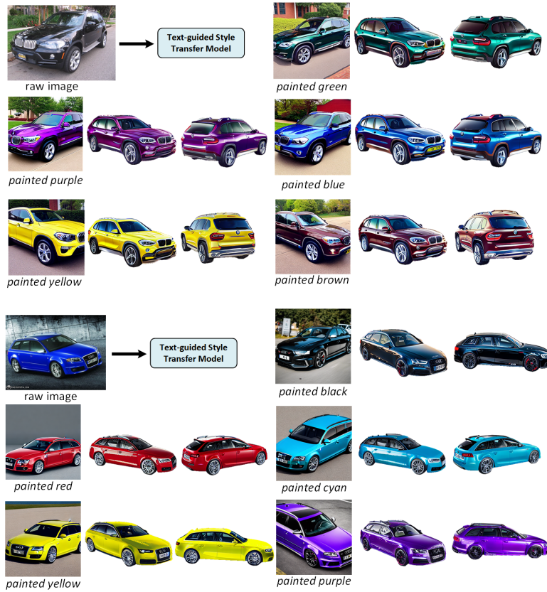
Fig. 13: We propose applying text-guided style transfer models [5, 19] to alter the vehicle’s paint in the raw image, utilizing prompts like "painted brown". Then, we use the proposed method to generate photorealistic renderings of the same vehicle model with different paintings.
