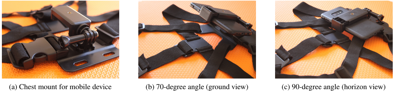
Figure 2: Chest mount for mobile device with adjustable collection angle settings.
