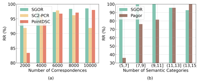
Fig. 6. (a): Registration Recall under different numbers of correspondences; (b): Registration Recall under different semantic conditions.
