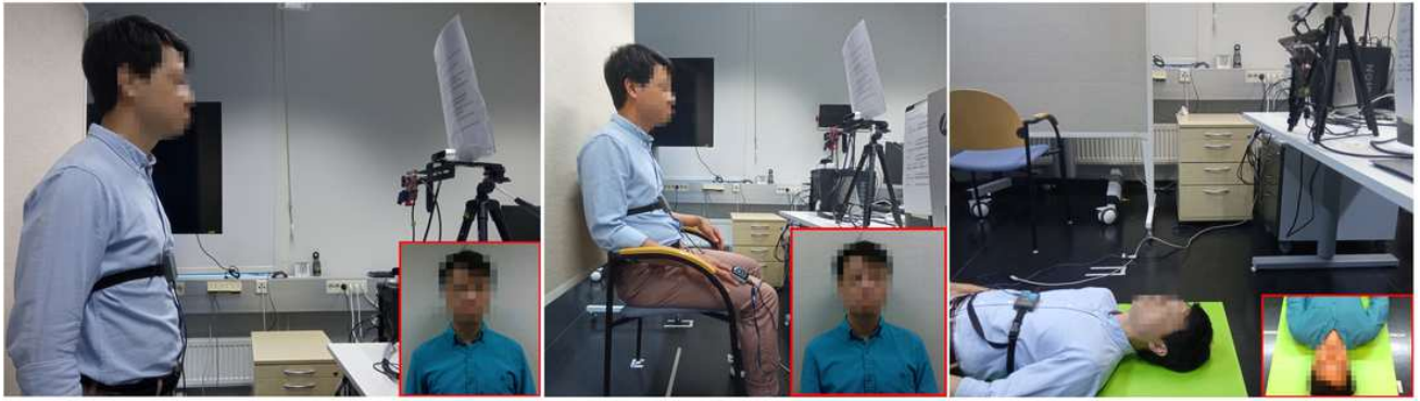
Fig. 5: Experimental setup for bio-movement radar analysis: Pose A (left) shows the subject standing 70 cm from the radar for breathing tasks. In Pose B (center), the subject is seated, with torso movement restricted by the chair, altering Doppler shifts. Pose C (right) has the subject lying down, executing the same tasks without torso constraints. The red square depicts the real image captured by the camera.
