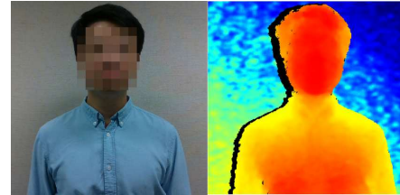
Fig. 2: RGB-D Camera stream: RGB data (left) and depth information (right).
