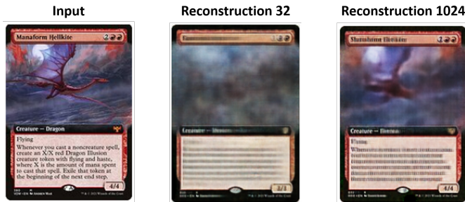
Fig. 3. Inputs and reconstructions of trained autoencoders. Input and outputs are of shape 3 \times 936 \times 672 , the latent spaces are 32-dimensional and 1024-dimensional respectively. The latent card representations are used as compressed input to the SNN (see Figure VI-A)
