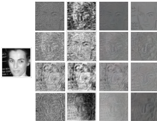
Fig. 5. Image restoration on a UNet reconstructed image. From top to bottom, target models are DCTDP, DLBPDP, HFCF-DLBP and Ours. The test image, results from UNet, results after applying the wiener filter and GFP-GAN are shown from left to right. The most right column contains the results from GFP-GAN when UNet reconstruct image without adding DP noise.
