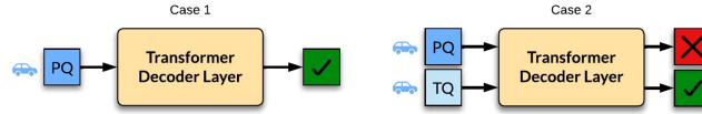
Fig. 4: An example of temporal confusion, where the decoder must handle the same proposal query differently based on the presence of track queries. In Case 1, the proposal query should be a positive prediction, while in Case 2, it should be a negative prediction.
