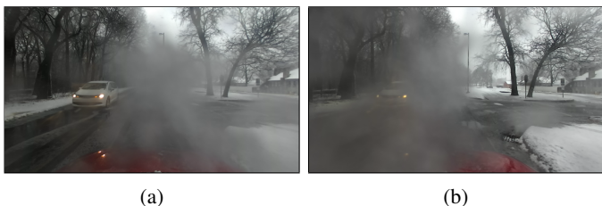
Fig. 6: A stereo image of the camera with lenses partially soiled by snow, represented by (a) the left and (b) the right images. This stereo image is extracted from sequence no. 26.
