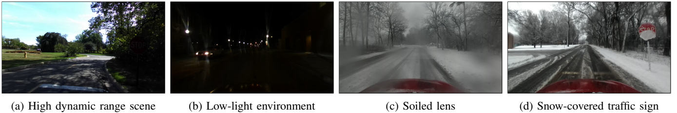
Fig. 7: Challenging scenarios represented in SID: (a) high dynamic range scenes, (b) low-light environments, (c) camera lens partially soiled by water droplets, and (d) snow-covered traffic signs.
