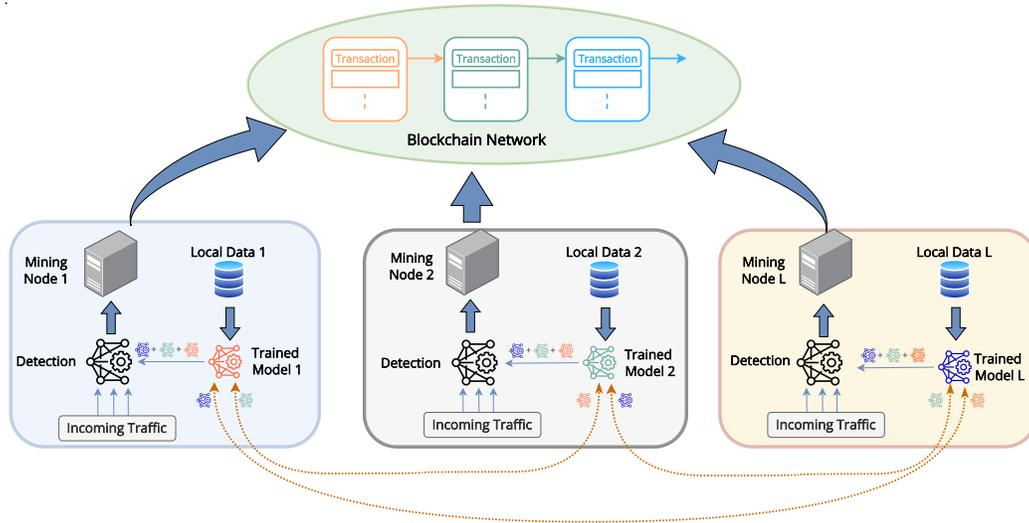
Fig. 1: Our proposed collaborative cyberattack detection model. The detection modules are first trained by their local data. They are then used to detect attacks for incoming traffic of blockchain networks before putting them into the mining nodes.
