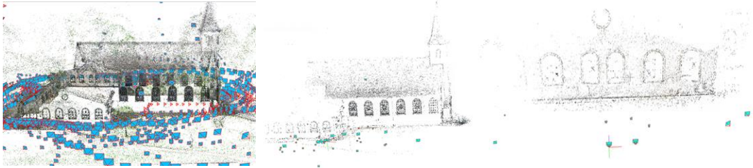
Figure 16. Reconstruction results of UniKirche . Left: complete reconstruction by v2. Middle and right: two sample sub-reconstructions by v1.
