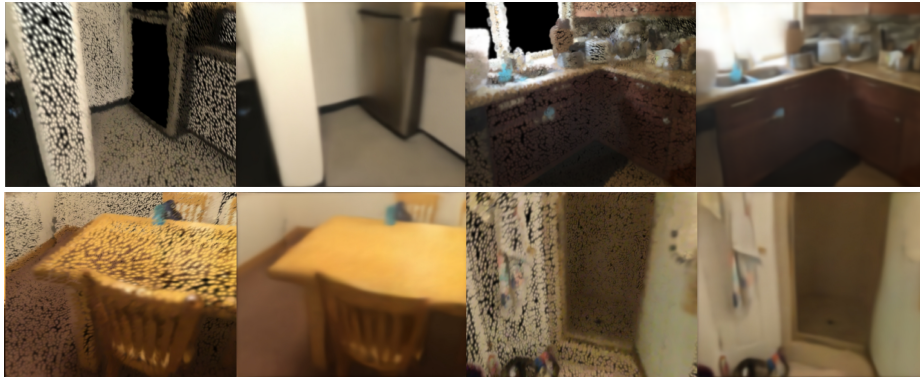
Fig. 9: Examples of point clouds containing large holes (row 1) and results with uneven density (row 2). The left side of each scene is the point splatting, and the right side is our method.
