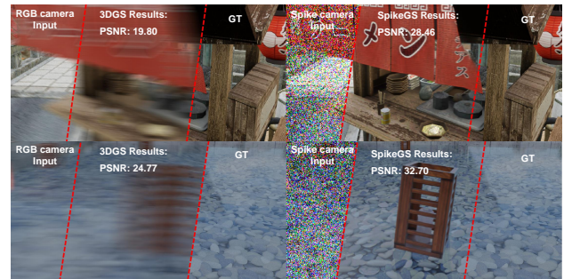
Figure 1: Brief introduction of SpikeGS. Given high temporal resolution but texture lacking spike stream captured by a fast-moving spike camera in one second , our method can reconstruct a sharp radiance field in minutes and achieves clear real-time rendering results.
