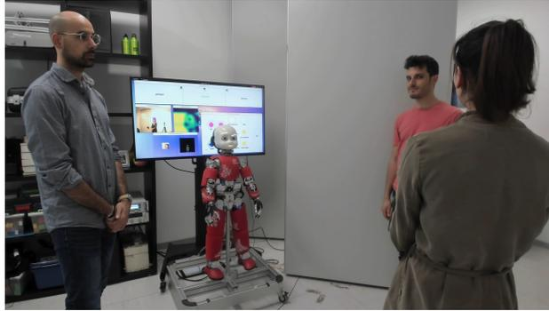
Figure 8: A frame of the multi-party conversation between the robot and the three actors. iCub is expressing a doubting face because it is estimating the addressee of the speaker in front of it; its LEDs are white because it has no role in the current dialogue. Behind the robot, we can see the visual explainability and transparency techniques (Figure 6).
