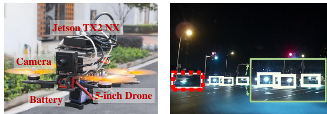
(a) Implementation of Anole on Jet- (b) Results in a typical night scen- son TX2 NX deployed on a UAV. nario.
