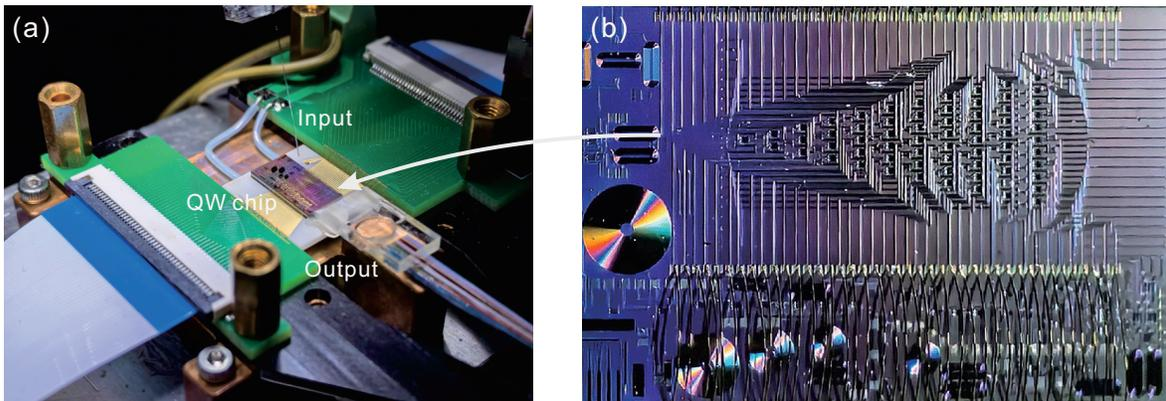
FIG. 4. **Experimental on-chip QWs and external setup.** (a) The experimental device includes a laser input connected to the photonic QW chip and an array of optical fibers coupled to the output ports. (b) A close-up view of the chip depicted in (a). The chip consists of 66 phase shifters, 78 beamsplitters, 24 input ports, and 24 output ports.
