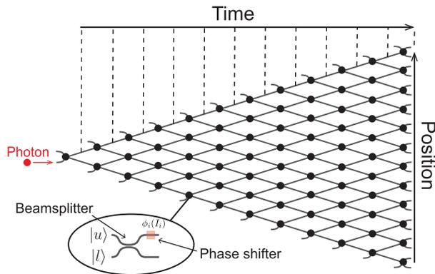
FIG. 2. **Conceptual diagram of the QW PIC.** Each black circle means a beamsplitter element followed by a tuneable thermo-optic phase shifter (see inset), and black solid lines represent the waveguides. At the last discrete time, the column of black circles represents only a beamsplitter without a following phase shifter, as it does not affect the output probability distribution.
