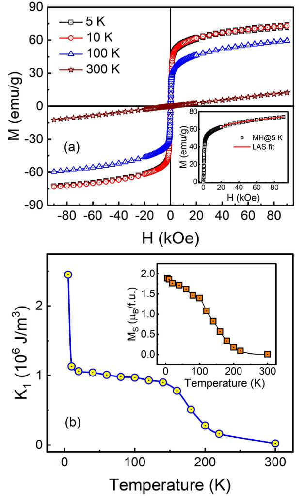
FIG. 3. (a) Isothermal magnetization as a function of applied magnetic field in the range  $\pm 90 \text{ kOe}$  at selected temperatures. Inset represents the virgin MH curve at 5 K along with the fit to the equation of law of approach to saturation (solid red line). (b) The temperature variation of cubic magneto-crystalline anisotropy  $K_1$  (solid blue line: guide to eye). Inset represents the saturation magnetization  $M_S$  as a function of temperature (solid black line: guide to eye).
