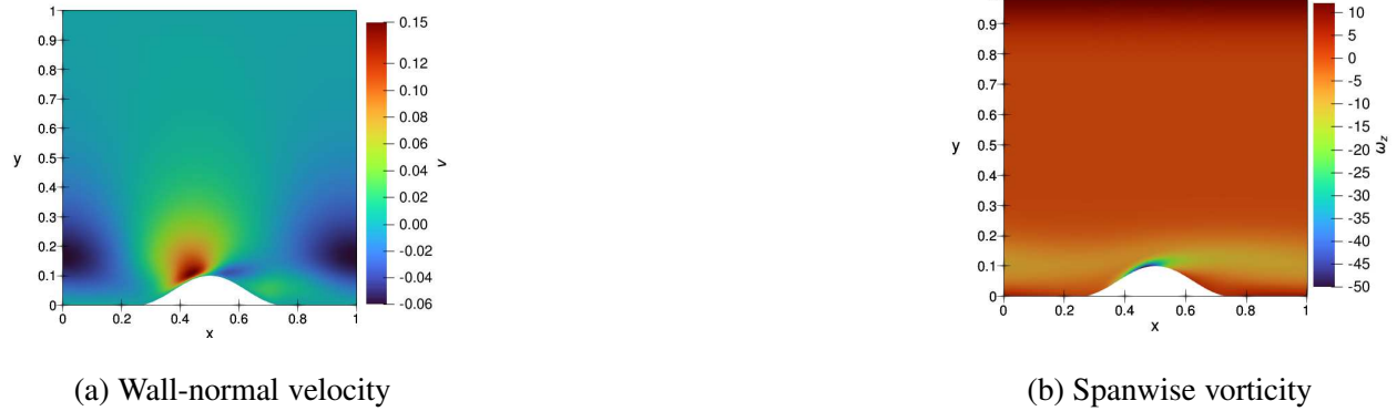
FIG. 3: Instantaneous (a) wall-normal velocity, normalized by U , and (b) spanwise vorticity field normalized by U/L_x , at spanwise plane z = 0.25 and time tU/L_x = 3.51 of local maximum drag
