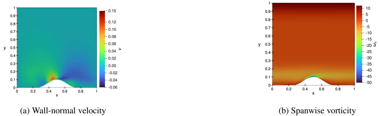
FIG. 4: Instantaneous (a) wall-normal velocity, normalized by U , and (b) spanwise vorticity field normalized by U/L_x , at spanwise plane z = 0.25 and time tU/L_x = 4.485 of local minimum drag
