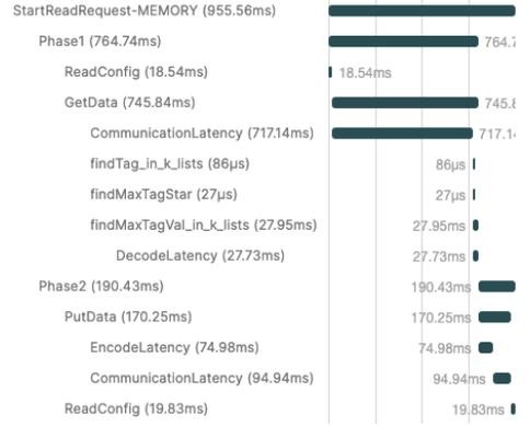
Fig. 4. READ Operation - algorithm: ARESEC, S:11, W:5, R:50, fsze:4MB, Debug Level:DSMM
