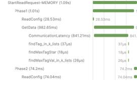
Fig. 7. READ Operation - algorithm: CoARESECF, S:11, W:5, R:5, fsze:512MB, Min/Avg Block Size:64MB, max Block Size:128MB, Debug Level:DSMM
