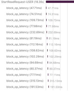
Fig. 5. READ Operation - algorithm: CoARESECF, S:11, W:5, R:5, fsze:512MB, Min/Avg Block Size:2MB, max Block Size:4MB, Debug Level:USER
