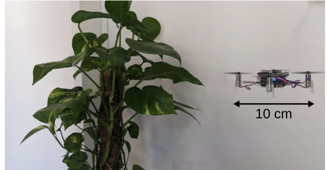
Fig. 1. Use case: a pocket-sized nano-drone inspecting a plant relying only on onboard sensing and computational capabilities.
