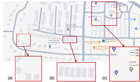
Figure 1: Illustrations of building multipolygon patterns for (a) houses, (b) townhouses, and (c) commercial buildings.
