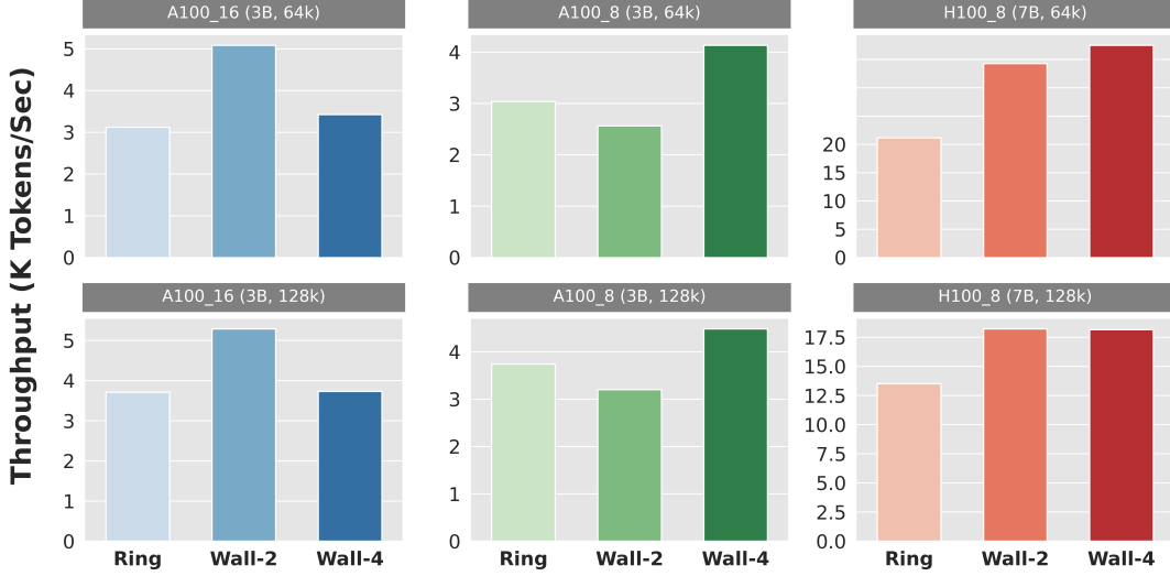
Figure 7. Throughput evaluation of Ring Attention and WallFacer on 32 GPUs from three different clusters. We place the performance of WallFacer with both C=2 and C=4 in the figure. The configurations are marked in the titles of the sub-figures. For instance, A100_8(3B, 63K) represents that the experiment is on machines with 8 Nvidia A100 GPUs in each node, the model used has three billion parameters, and the sequence length is 64k.
