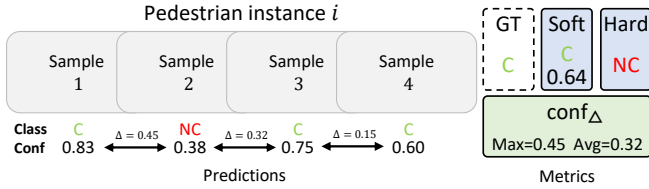
Fig. 4: Per-instance metric example for binary action prediction. GT refers to ground truth. Soft label is computed by averaging over prediction confidence of all samples. Hard label is set to a label other than ground truth if prediction for at least one sample does not agree with the rest, i.e. it is treated as a misprediction. If predicted labels for all samples are the same, hard label will be the same.
