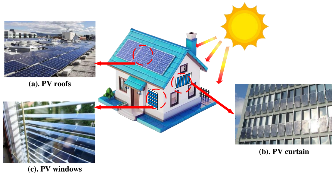
Figure 4. Three types of BIPV were assessed in this work.
