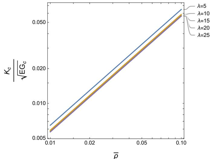
FIGURE 3. Zeroth-order homogenized octet frame. Dependence of normalized mode-I toughness  $K_{c,0}/\sqrt{EG_c}$  on relative density  $\bar{\rho}$  and slenderness  $\lambda$  of the bars.
