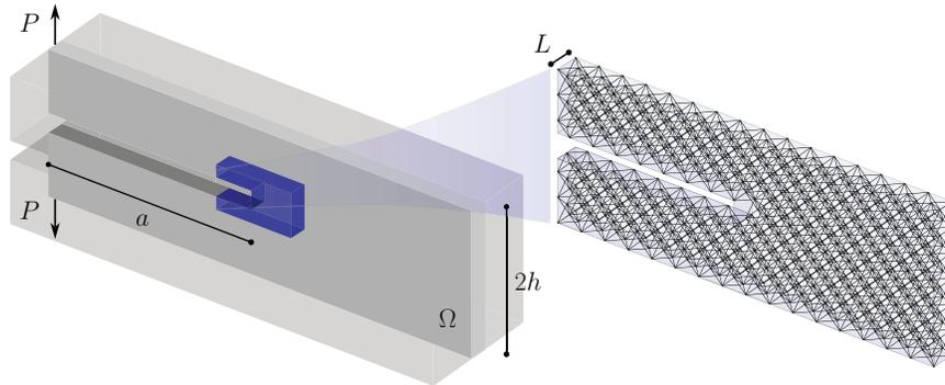
FIGURE 4. Octet-frame metastructure, double-cantilever beam configuration.
