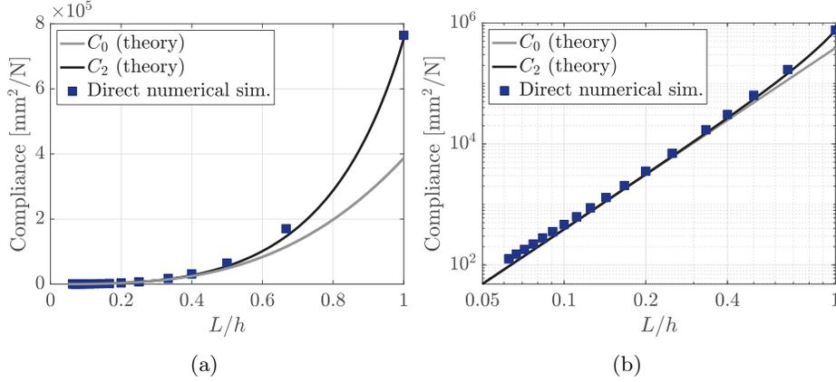
FIGURE 5. Octet-frame metastructure,  $EA = 1.43$  N,  $EI = 3.77 \times 10^{-4}$  N mm<sup>2</sup>,  $L = 0.75$  mm. Double-cantilever plate configuration,  $a = 48$  mm,  $h \in [0.75, 12]$ . Compliance as a function ratio  $L/h$  of cell size to plate thickness. Comparison of direct calculation using a bar model, zeroth-order continuum limit (76) and second-order continuum limit (84). (a) Linear plot; (b) log plot.
