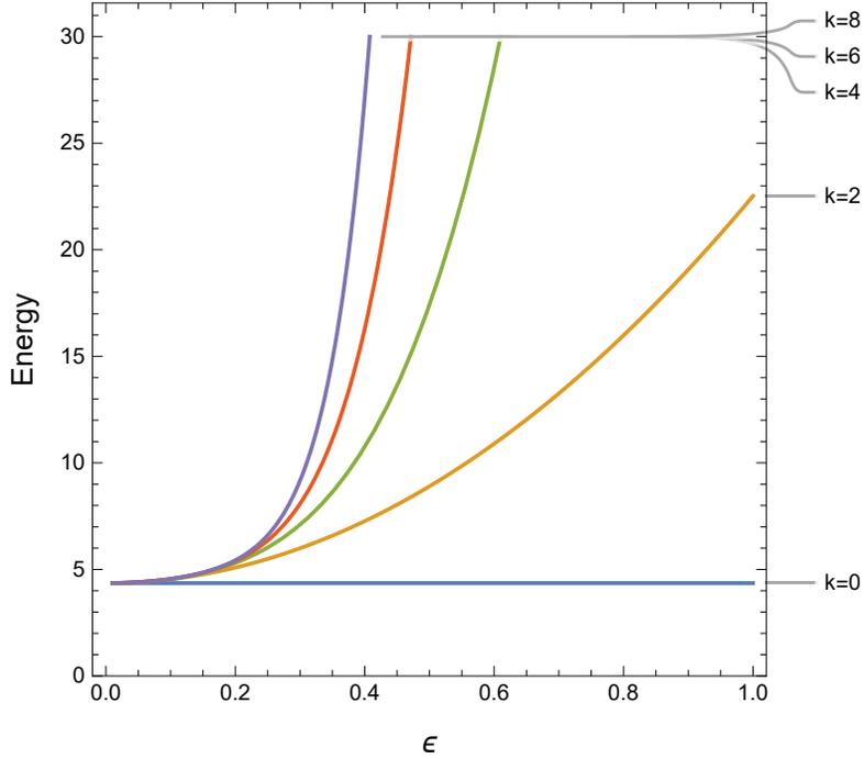
FIGURE 2. Dipole in octet metamaterial constrained to deform in uniaxial strain.  $\Gamma$ -expansion of normalized energy to order  $k = 0$ .
