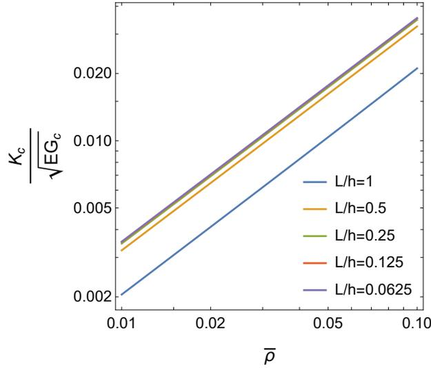
FIGURE 6. Second-order homogenized octet frame. Dependence of normalized apparent mode-I toughness  $K_c(a, L)/\sqrt{EG_c}$  on relative density  $\bar{\rho}$  and size  $L$  of the unit cell for long cracks  $a \rightarrow +\infty$ .
