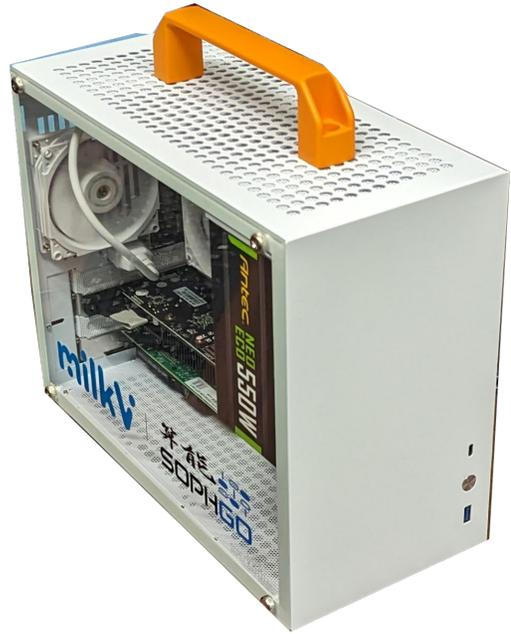
Fig. 1: Image of one of the MILK-V Pioneer nodes of the in-house cluster. Each node has a 64-core SOPHON SG2042 RISC-V CPU and 128 GB DDR4 System Memory. The colorscheme of box (the orange handle and white case) reminded us of the snowman Olaf from the movie Frozen. For this reason, we named the cluster Olaf ☺.
