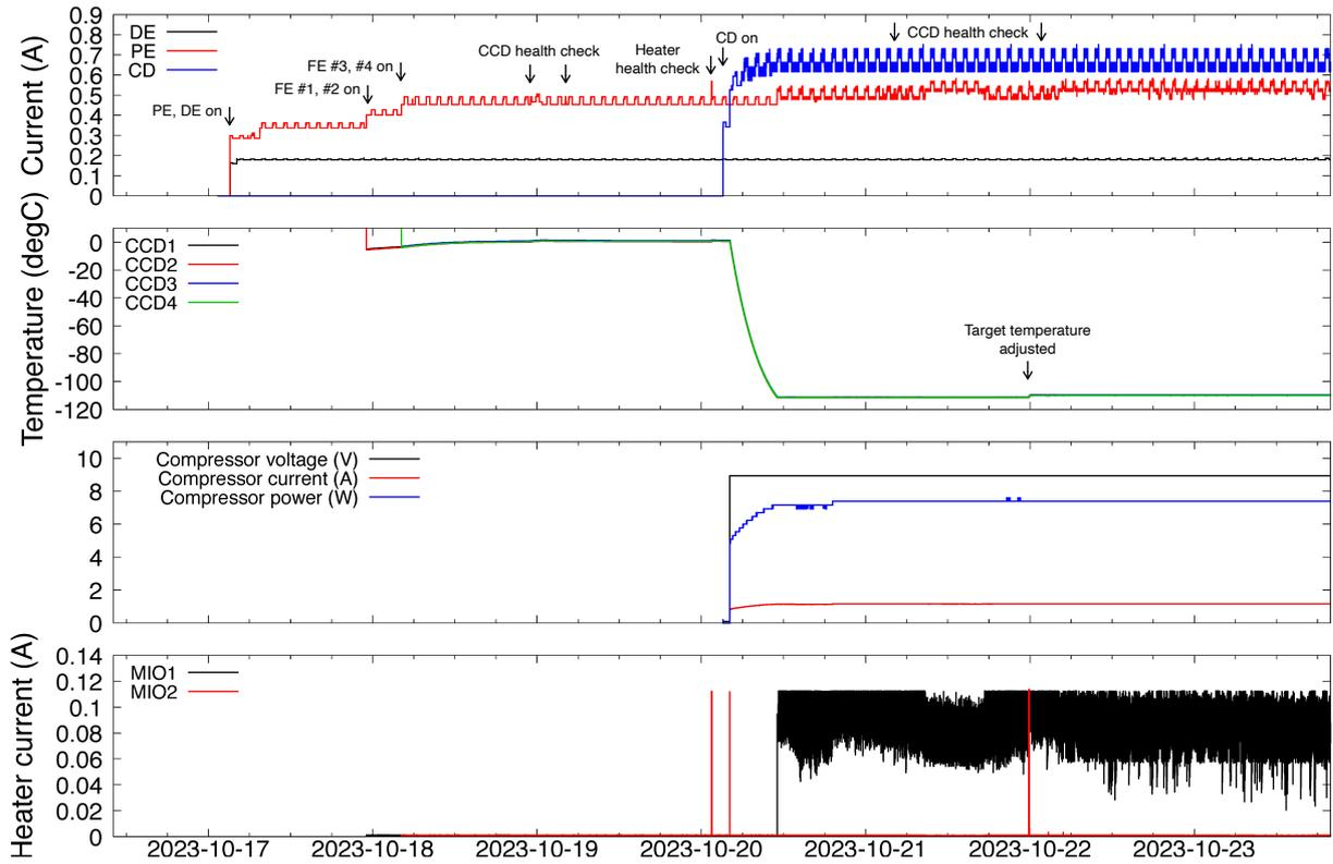
Figure 1. Timeline chart of the SXI house-keeping data related to the electronics and cooling system during the start-up operations.
