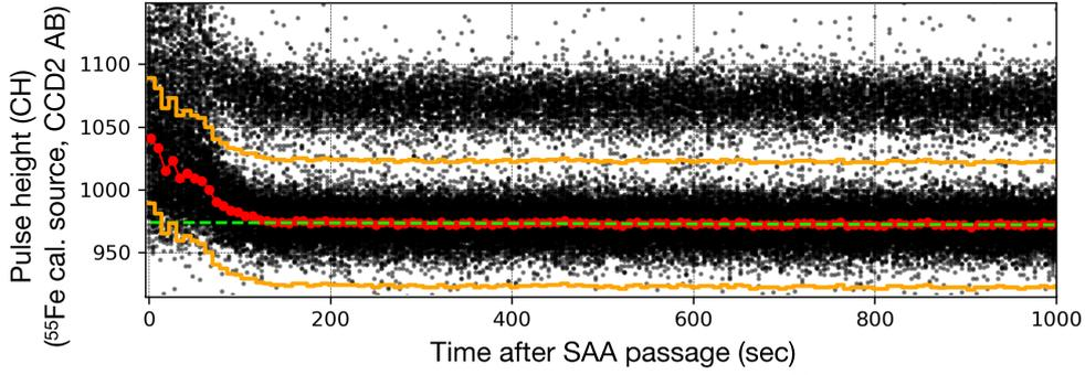
Figure 4. Behavior of pulse heights of Mn-K $\alpha$  and K $\beta$  X-ray events from the  $^{55}\text{Fe}$  calibration source after SAA passages. The black dots are X-ray events. The green dashed line indicates the average pulse height of Mn-K $\alpha$  in the stable period. The Mn-K $\alpha$  centroids at individual time bins, calculated from the data points enclosed with the orange lines, are shown in red.
