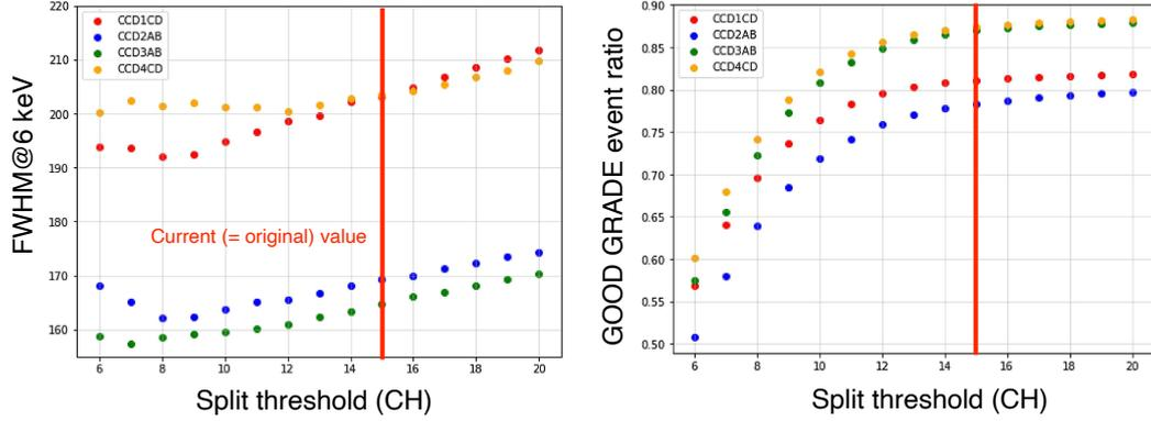
Figure 6. Split-threshold dependence of spectroscopic performance, the energy resolution (left) and good-grade event ratio (right). The red vertical lines are the original value of the split threshold determined before the launch, which was kept unchanged. The energy resolution in the left panel is less than the full performance<sup>7</sup> because we used data before the full processing.
