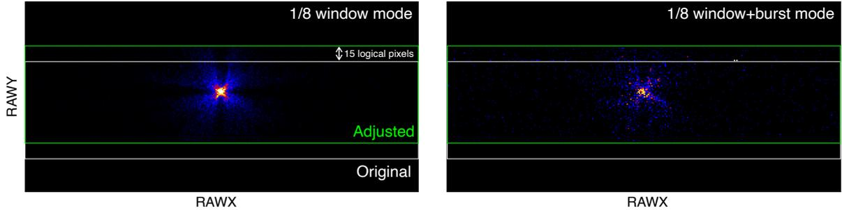
Figure 7. Point-source images obtained with the 1/8-window (left) and 1/8-window+burst (right) modes after the adjustment of the window position. The white and green boxes indicate the window regions before and after the adjustment, respectively.
