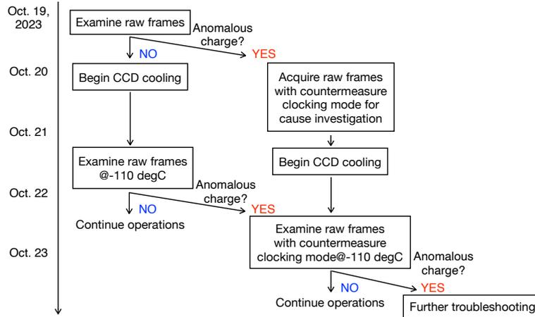
Figure 3. In-orbit operation procedure against the anomalous charge problem. In reality, we did not experience the anomalous charges, and thus we followed the simplest (leftmost) case.
