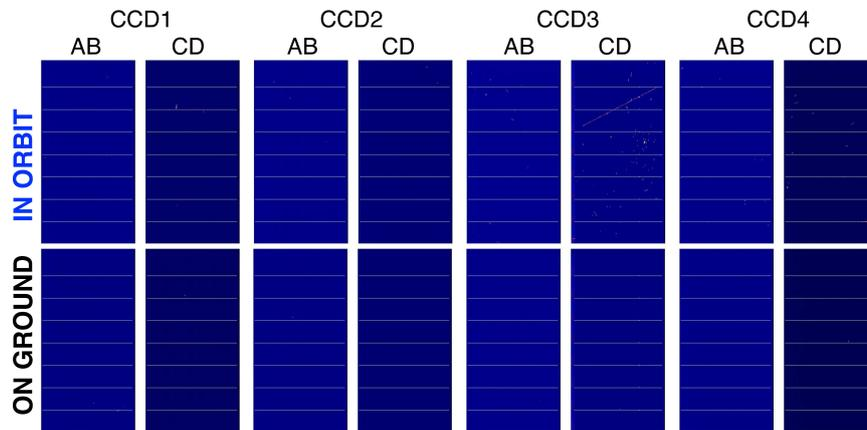
Figure 2. In-orbit raw frame images at  $-110^{\circ}\text{C}$  and a comparison with on-ground frames. The eight white rows in each frame are the charge-injection rows, where the pulse heights are saturated at 4095 ch. The color scale is the same for all the frames (0–4095 ch). The white dots and tracks seen in the in-orbit frame images are cosmic-ray induced events.
