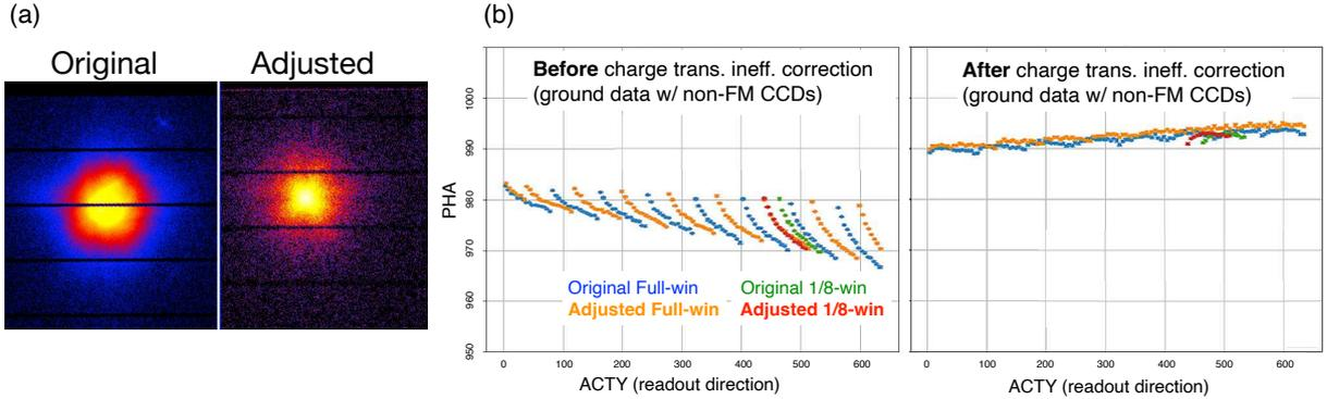
Figure 8. (a) Extended-source images before and after the charge-injection-row adjustment. The black rows without counts are the charge-injection rows. (b) 5.9 keV pulse height distribution along the readout direction before and after correction for charge transfer inefficiency. These are from on-ground experiments to confirm that the original charge-transfer-inefficiency correction algorithm is applicable to the data obtained after the adjustment of the charge injection rows.
