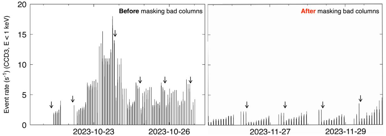
Figure 5. Event rate of CCD3 during night-earth observations before and after masking bad columns. The black arrows indicate time at which dark levels were initialized.
