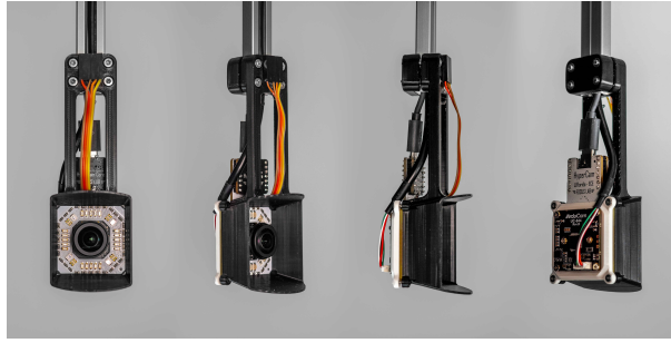
Fig. 2. The same components can fit into a minirhizotron with a dedicated case design.
