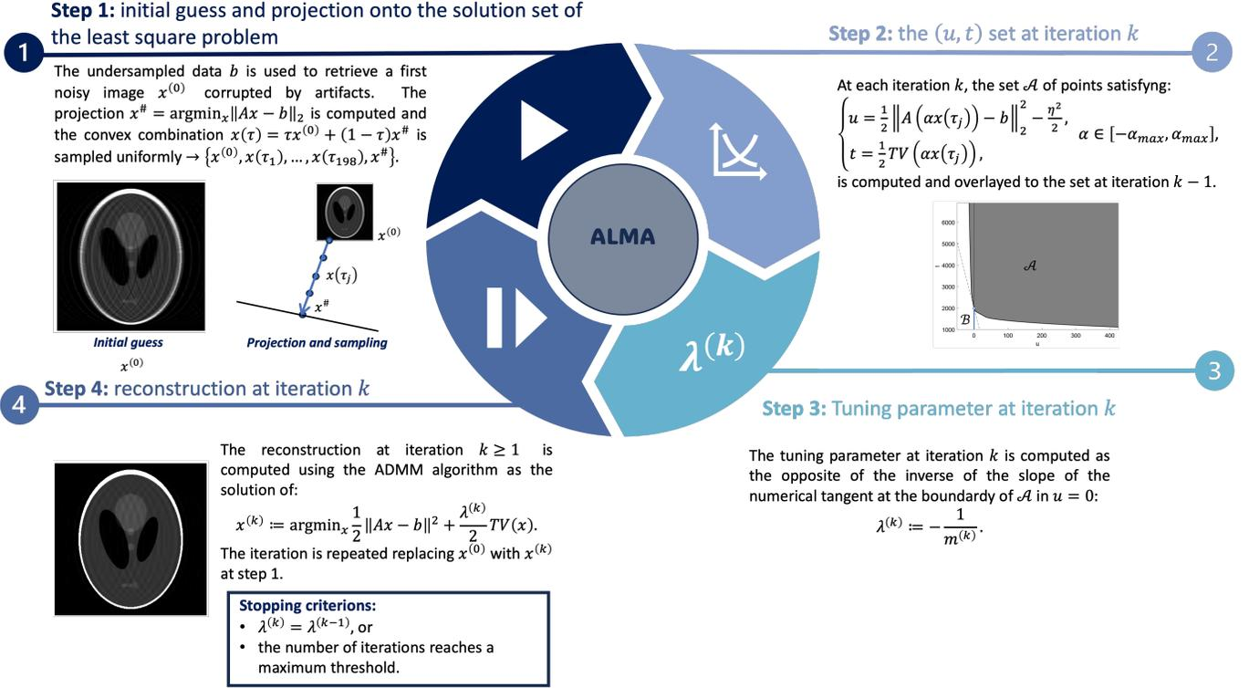
Fig. 4: Schematic representation of ALMA.
