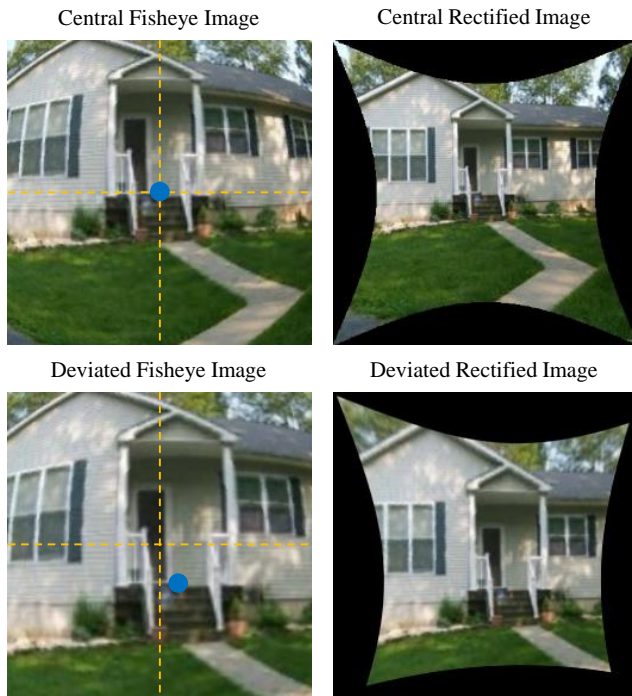
Figure 1: Examples of a central fisheye image and a deviated fisheye image, together with their rectified images.
