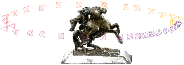
Fig. 6. Cycle graph 3D reconstruction with 38 poses. Rotation averaging using the primal-dual algorithm (1) takes 2ms. For reference, our implementation of the closed-form solution takes 0.07ms.
