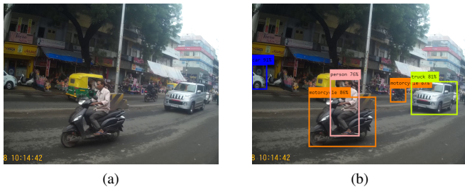
Fig. 4: A real-world road traffic scenario [1] and the corresponding object detection provided by YOLO trained on the COCO dataset [10].
