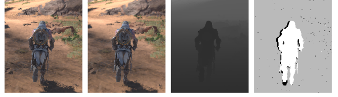
Fig. 7. The inputs of shading correction network (SCN). Images from left to right are: the output of GAE module \tilde{J}_{t+\alpha}^{\text{GAE}} , the backward warped result I_{t-1 \rightarrow t+\alpha}^w from frame t-1 using motion vectors, the generated depth buffer \tilde{D}_{t+\alpha} , and the input mask M_t^{\text{input}} .
