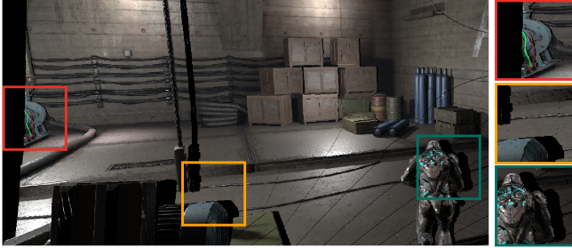
Fig. 2. An extrapolated frame by directly projecting fragments from previous rendered frame. The right column shows three types of disocclusions: out-of-screen disocclusion , static disocclusion and dynamic disocclusion from top to bottom. The thin black lines splatted in the image are due to forward warping.
