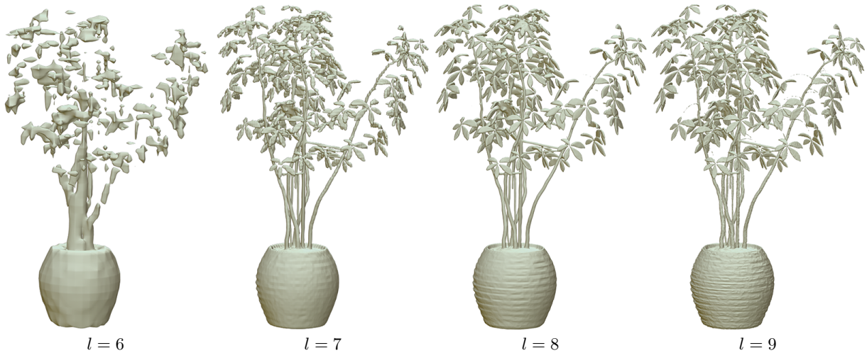
Figure 3: Qualitative results from octrees spanning level 6 to 9. As the resolution of the octree increases, it provides more degrees of freedom, effectively improving the quality of the reconstructed geometry.
