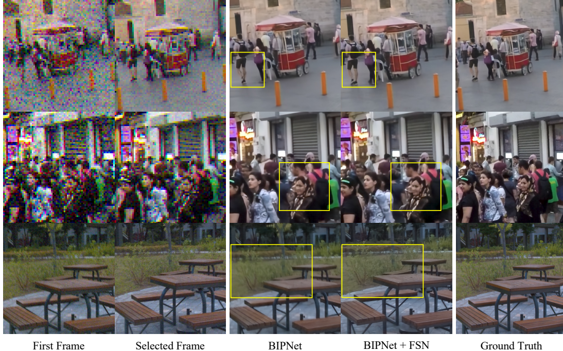
Figure 5. Qualitative comparison on synthetic-NEBI (top two rows) and real-NEBI (bottom row). BIPNet [11] with our frame selector enhances high-frequency image details by merging effectively complementary information from multiple frames into the selected base frame, while BIPNet [11] predicts blurry images due to the severe degradations in the first frame. Best view to zoom.
