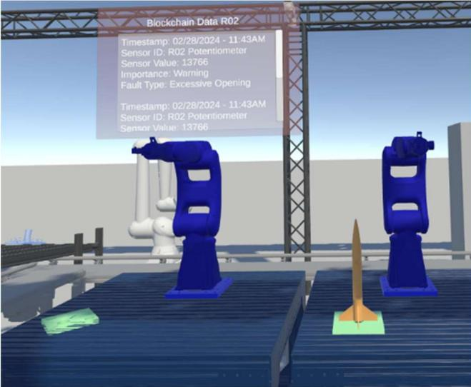
**FIGURE 9:** VISUALIZATION OF FAULTY DATA FOR INDIVIDUAL ASSEST RETRIEVED FROM THE BLOCKCHAIN DATABASE
