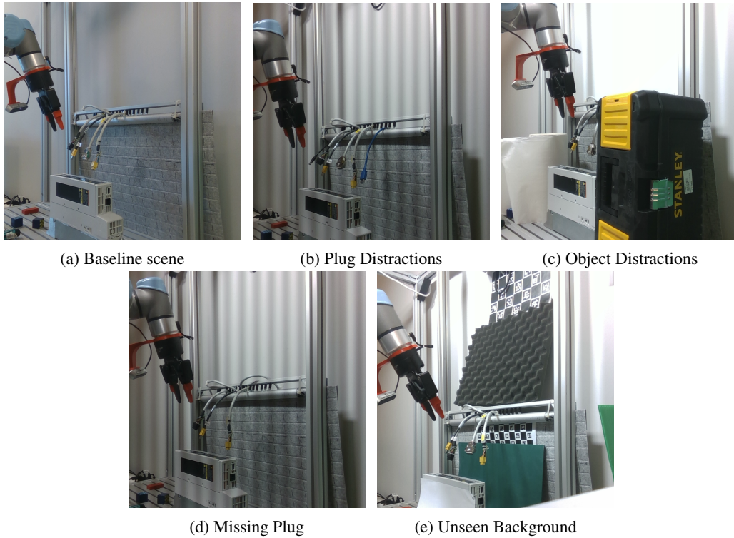
Figure 3: Examples of perturbations introduced in the experimental setup to evaluate the robustness of our model. Each sub-figure illustrates a different type of perturbation.
