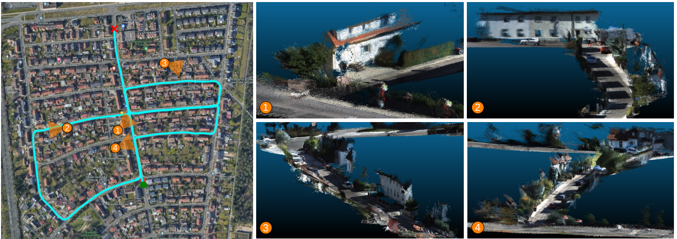
Figure 14. iSLAM tracks the robot’s trajectory (left) in real-time and simultaneously performs a dense reconstruction (right 1-4).
