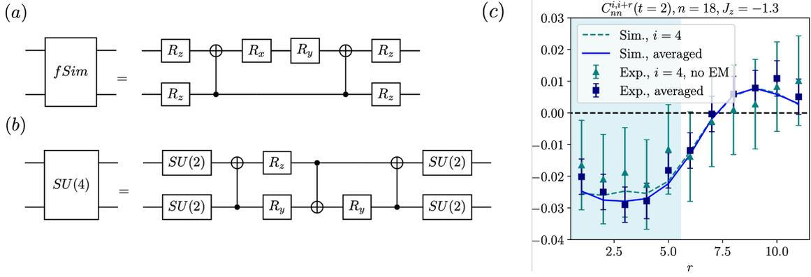
Figure 7. Synthesis of the (a) fSim gate and (b) SU(4) gate into CNOT and single-qubit gates. Each CNOT gate can be further decomposed into single-qubit rotation gates and exactly one  $R_{ZZ}$  gate native to the Quantinuum’s QCCD processor. (c) Comparing the density-density correlation function between averaged over the bulk sites and simply setting the initial site at  $i = 4$ .
