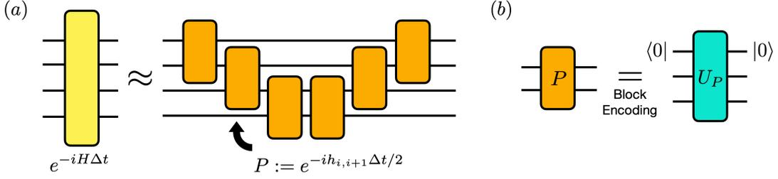
Figure 8. (a) A Trotterization ansatz considered in Appx. C  $e^{-iH\Delta t}$  is approximated by a series of ladder-shaped nearest neighbor time evolutions  $P$ . (b) To implement a non-unitary operation, the typical way is to implement  $P$  in a unitary,  $U_P$ , in doubled Hilbert space and postselected on the ancilla qubit getting 0 outcome.  $U_P$  can further be synthesized into local unitary circuits with, e.g., SU(4) gates.
