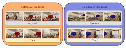
Figure 2: Gaussian Splatting dataset sample trajectories. The trajectories are designed in two phases, first an approach where the drone gets close to the target and centers it in the middle of the image, followed by a turn procedure in the direction corresponding to the color of the target.
