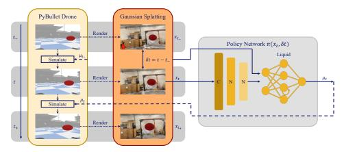
Figure 3: Diagram of the in-simulation inference protocol with physics engine dynamics and GS rendering. At time t, the GS image  $x_t$  is rendered from the simulated position and attitude, and processed through the CNN of the policy network  $\pi(x_t)$ . Obtained features, along with the elapsed time  $\delta t = t - t_-$ , are input into the Liquid network, which outputs the velocity control command.
