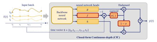
Figure 9: Liquid (Closed-form Continuous-depth) neural architecture. A backbone neural network layer delivers the input signals into three head networks g, f, and h. f acts as a liquid time constant for the sigmoidal time-gates of the network. g and h construct the nonlinearities of the overall CfC network. (Adapted from [6] with the authors' permission.)
