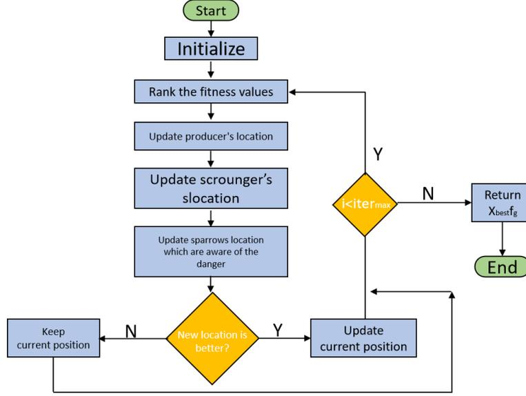
Figure 4. Flow chart of the SSA model
