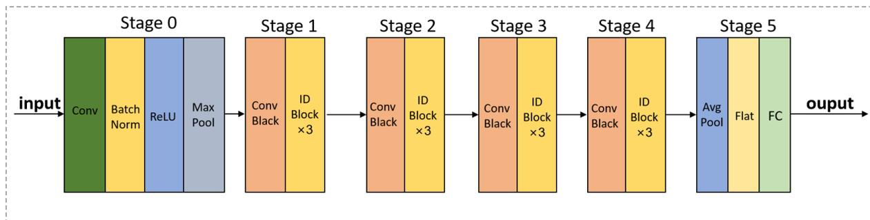
Figure 2. Flow chart of the ResNet50 model
