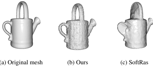
Figure 4. Visualization of mesh reconstructions of Can object in LM. The figure shows the original mesh, our reconstruction from NeRF using marching cubes, SoftRas refers to mesh optimized using SoftRas differentiable renderer. SoftRas mesh cannot reconstruct holes as it is optimized from genus zero sphere mesh.
