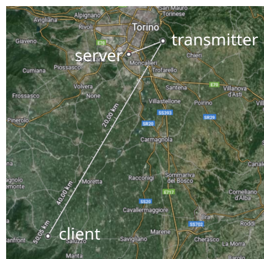
Figure 6: map of client, server and transmitter for test with the client at a remote site.
