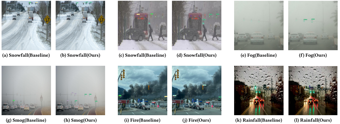
Figure 2: Comparison of YOLO v8 tested for naturally occurring real images. Left: Images tested on model fine-tuned on the proposed pipeline for artificial snow dataset. Right: Images tested on model model fine-tuned on ground truth traffic light dataset
