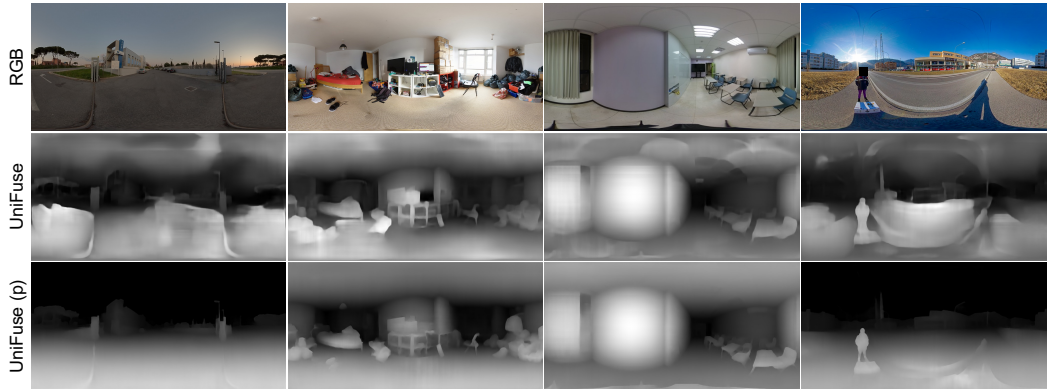
Figure 6: Generalization ability in the wild with depth map visualization: We showcase zero-shot qualitative results using a combination of images captured by us and randomly sourced from the internet to assess the model’s generalization ability. For privacy reasons, we have obscured the camera-man in the images.
